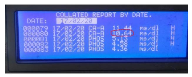
READING SHOWN IN THE MACHINE FOR THE IQC CALCIUM SAMPLE 17/02/2020
