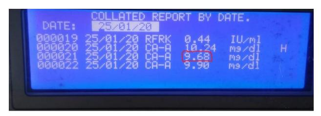
READING SHOWN IN THE MACHINE FOR THE IQC CALCIUM SAMPLE 25/01/2020
